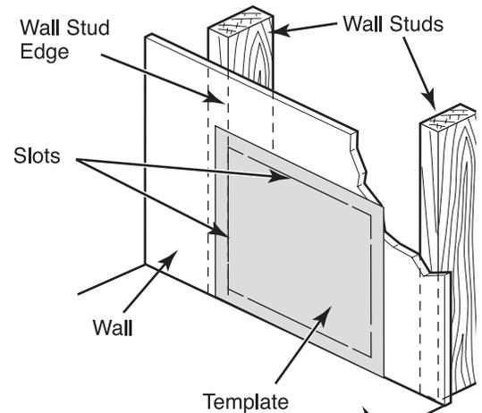
2. Use a utility knife to carefully cut inside the penciled outline area. Start with the stud side and work outward. **DO NOT USE A SAW.** Remove sheet rock section to expose **wall cavity**. Bring **water** and **power supply** lines from source to this location. Allow 18" of slack. **See Figure 2.**
